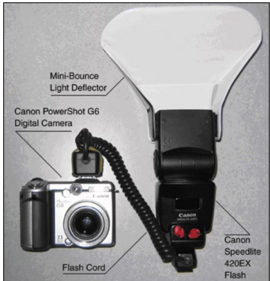
Figure 2. Ideal Photographic Setup for Documenting Assembly Procedures
